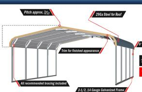
\*BUILDINGS OVER 35' L RECOMMENDED TO GO ALL VERTICAL (Due to Engineering Specifications; to avoid leaking.)
